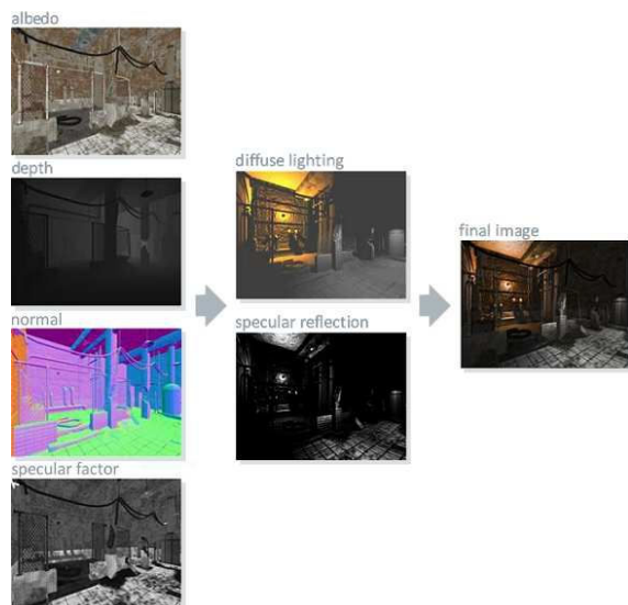
Figure 4: An example overview of different passes applied to a deferred shading pipeline. (Leadwerks, 2008).
